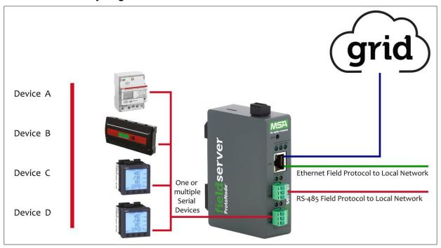
The ProtoNode can connect with the MSA Grid – FieldServer Manager. The FieldServer Manager allows technicians, the OEM's support team and MSA Safety's support team to remotely connect to the ProtoNode. The FieldServer Manager provides the following capabilities for any registered devices in the field:
