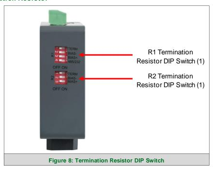
If the ProtoNode is the last device on the serial trunk, then the End-Of-Line Termination Switch needs to be enabled. To enable the Termination Resistor, move the TERM dip switch to the right as shown in Figure 8.
